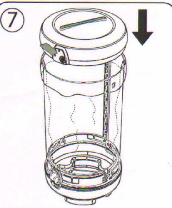
With the key still in position, offer the hood onto the body aligning with the rear bobbin. When aligned turn hood clockwise then remove key.
