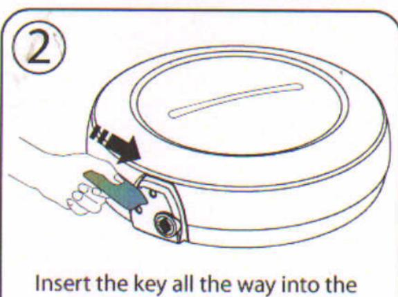
lock. (Do not turn the key.) This will automatically release the locking mechanism.
